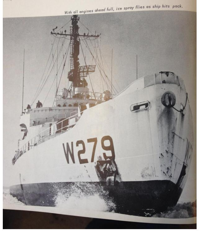
Specially constructed bow allows ship to easily ride up on ice.
